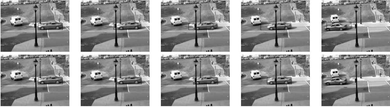
Figure 6. Frames 1, 2, 5, 10, 20, and 30 of a sequence with an occluder. Top row: The adaptive mean shift tracker wanders significantly. Bottom row: The illumination invariant tracker formulation maintains a lock on the car while it passes behind the occluding lamppost.
