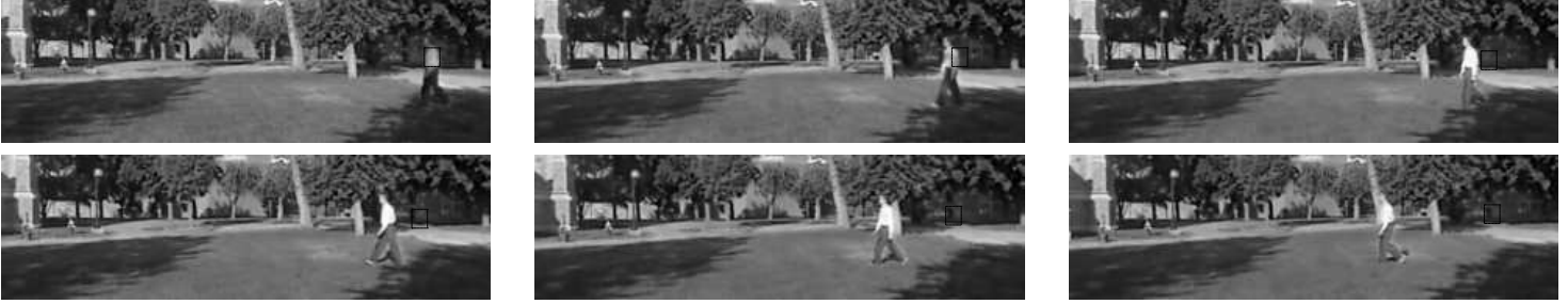
Figure 4. Results of using the adaptive mean shift tracker for a sequence with strong shadows. The figure shows frames 1, 10, 20, 30, 50, and 70. The tracker begins to lock onto the darker background (and fails to recover) as the subject moves into an area of strong lighting.
